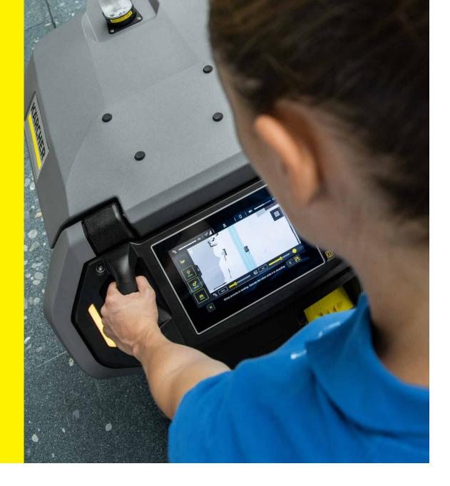
and using manual cleaning mode. The display always shows the buttons required for the current task only – making it simple and safe. Even the surroundings detected by the sensors can be visualized using a map during set-up, so that you can see even more precisely what the cleaning robot detects and where it has already cleaned.
