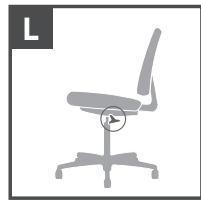
L. Tilt lock — Locks out tilt function.
