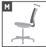
M. Posture mechanism/lock — Back angle adjusts independently of seat, and can be locked in an infinite number of positions within a fixed range.
